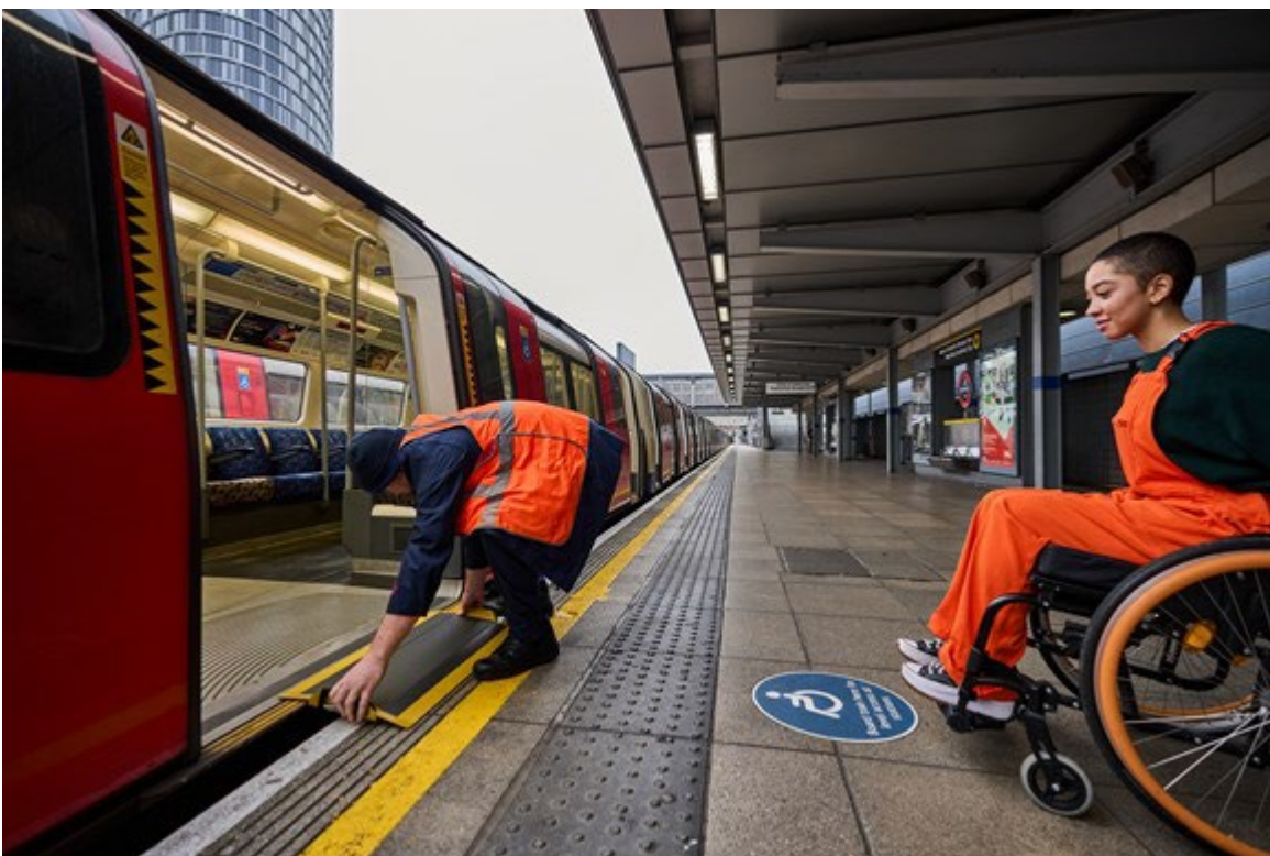
Figure 40. Accessibility bridging device being used on the Tube network during the trial. Source: TfL.
